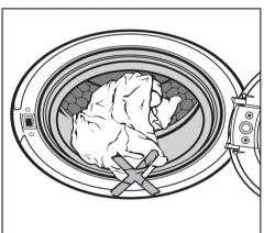
To prevent damage to the door seal and clothing, make sure that there is nothing caught between the drum door and the seal.
